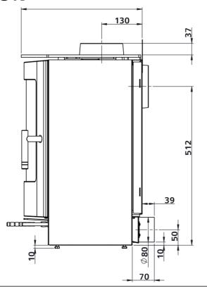
The direct air intake spigot (80mm diameter) to the rear ofthe appliance is removable with a 2.5mm Allen key.
