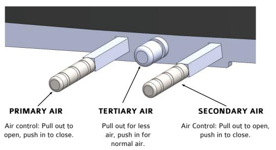
Air regulation, the three control levers perform differing tasks in regulating the combustion air on your appliance:
