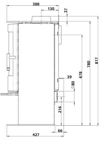
\*\* The additional, top flue rear convection panel (supplied loose within the stove) needs to beused when installing the stove 100mm from a combustable wall; this slots over the rear convection panel and provides additional radiant protection from the flue collar.
