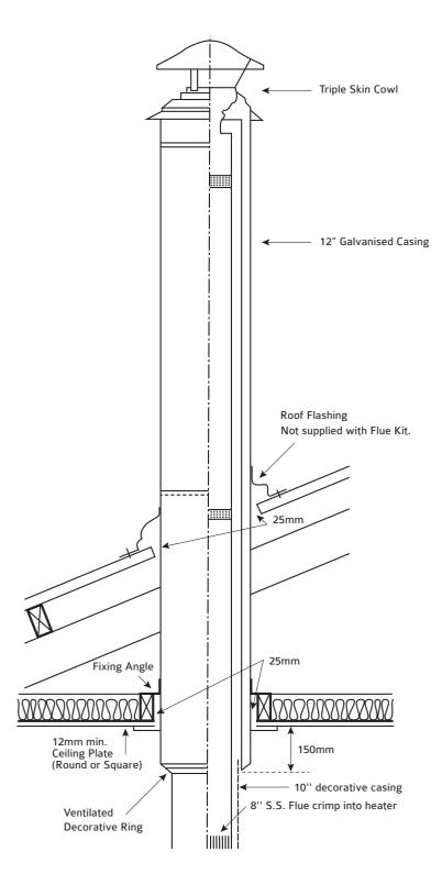
The following drawings are meant as a guide only. Your wood heater must be installed by a qualified person whose work conforms with local council regulations, Australian/ New Zealand standards (AS/NZS 2918:2018) & manufacturers recommendations.
